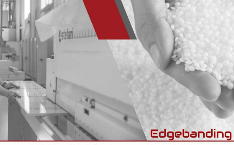
Due to their flexibility and high adhesion performance, Hotmelt (EVA based) adhesives are frequently used in edge banding applications in the furniture industry.
